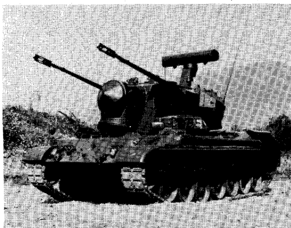
Fig. 18. Flakpanzer AA tank for the Dutch army, showing X-band search radar antenna on top and combined X- and Ka-band tracking antenna at the front of the turret (photo courtesy Hollandse Signaalapparaten).
